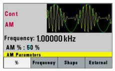
Both models provide AM and FM modulation along with linear/logarithmic sweep and built-in counter capabilities. Internal and external sources can be used for triggering and modulating the signal.
