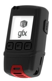
The EL-GFX-1 standalone USB data logger measures and stores up to 256,000 temperature readings over a -30 to +80°C (22 to +176°F) range and at a resolution of 0.1°C. Using the Windows control software (available as a free-download from www.easylogusb.com), users can quickly set up the data logger and view downloaded data by connecting the device to the PC's USB port using the supplied cable.
